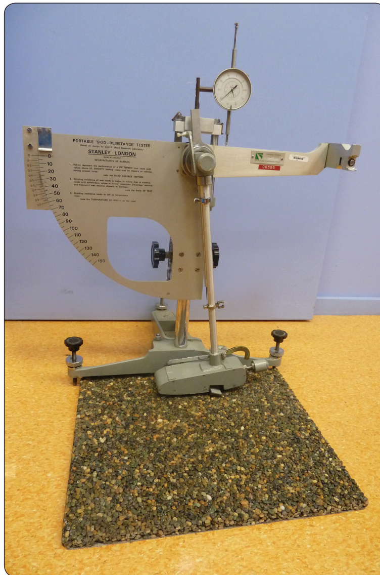
Figure 2. The pendulum CoF test (also known as the portable skid resistance tester, the British pendulum, and the TRRL pendulum).
